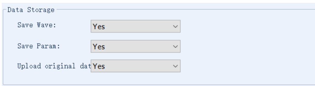
Fig. 8-1 Data Storage configuration for Qingcheng IoT Cloud
