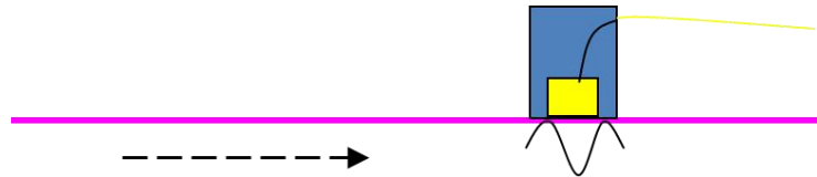
Fig. 3-14 Schematic diagram of surface wave received by sensor
