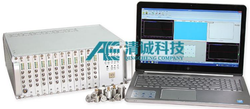
Fig. 3-1 SAEU3H digital acoustic emission testing system
