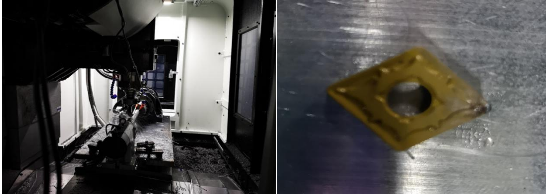
Acoustic emission monitoring site of tool wear during machining
