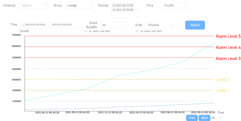
Figure 2:1 Multi-channel Counts display of tower No. 1
